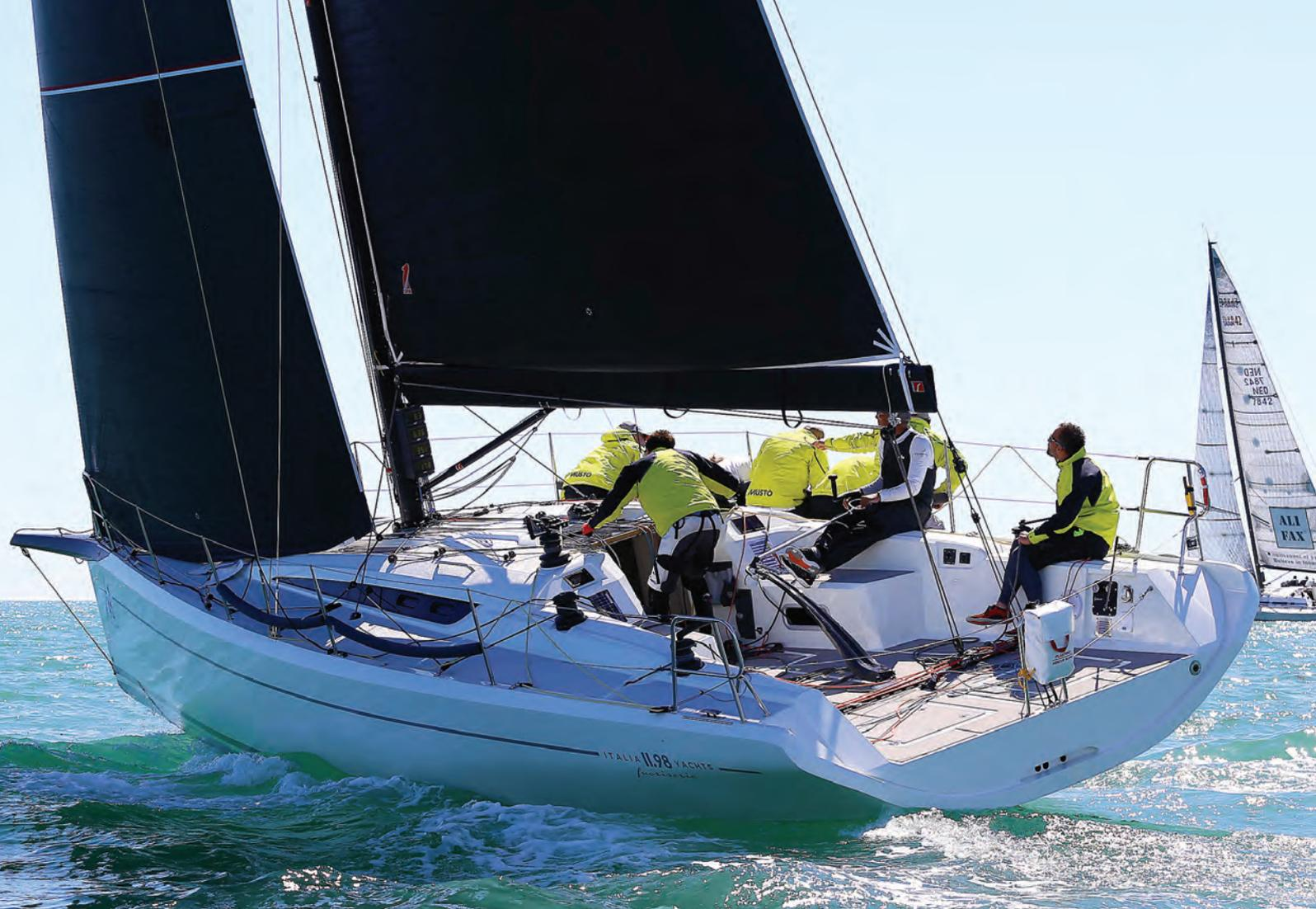
**The ends of the 11.98 have been drawn in at the waterline relative to its smaller predecessor to take away some wetted surface and improve performance in light airs. At the same time, as well as adding stability and power, fuller mid-sections combine with the finer ends to allow the boat to be very easily trimmed fore and aft, giving the crew more flexibility than a higher-prismatic design would**
